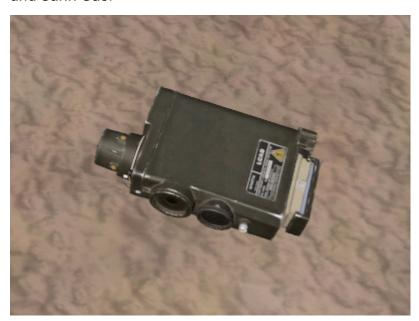
• Man-Portable Chemical Agent Detector (MCAD) - Detects Liquid Nerve Agents, Mustard Gas, Chlorine Gas, and Sarin Gas.
