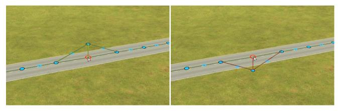
Image-7: Positive and Negative Elevation Changes for a Road
