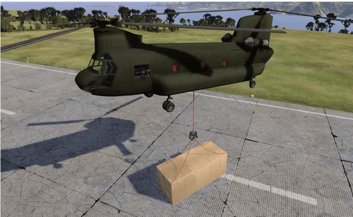
Ropes can be created and controlled via CIGI packets. For more information, see **Entity Rope Control Component Control** in the [online ICD Reference](https://manuals.bisimulations.com/cigiicd/icd_23_2/index.html) ([https://manuals.bisimulations.com/cigiicd/icd\\_23\\_2/index.html](https://manuals.bisimulations.com/cigiicd/icd_23_2/index.html)).
